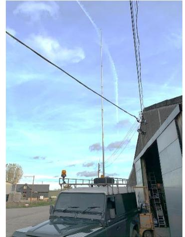
4. As part of regular testing our Clark Mast has been erected to test out that its seals and locking nuts are OK. This confirmed that it is fit-for-purpose.
